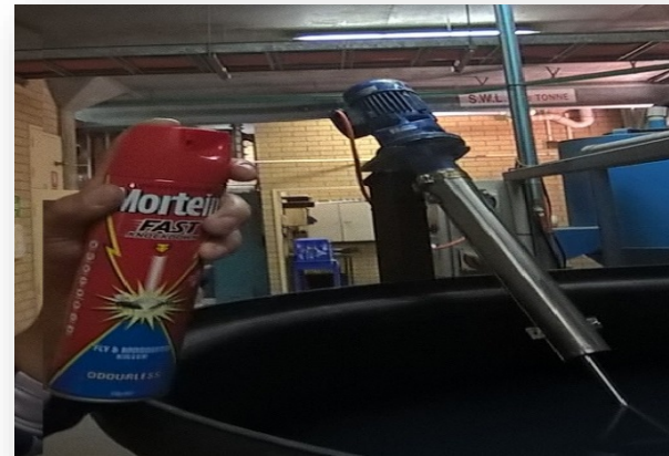
Spraying pests in close proximity to a water treatment process
