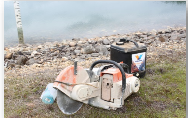
Filling up equipment directly next to a water storage without adequate spill control - note the lid left off the oil container
