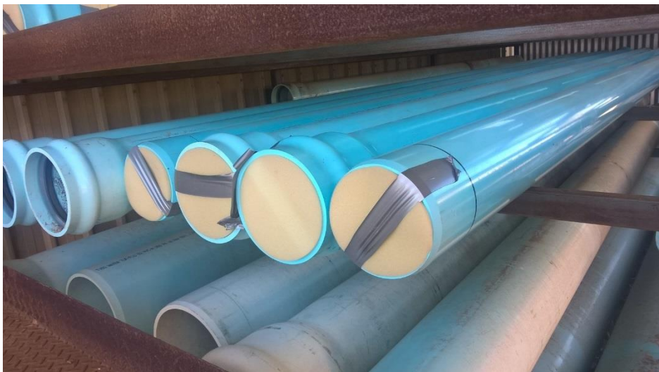
A simple solution to avoid the entry of contaminants
