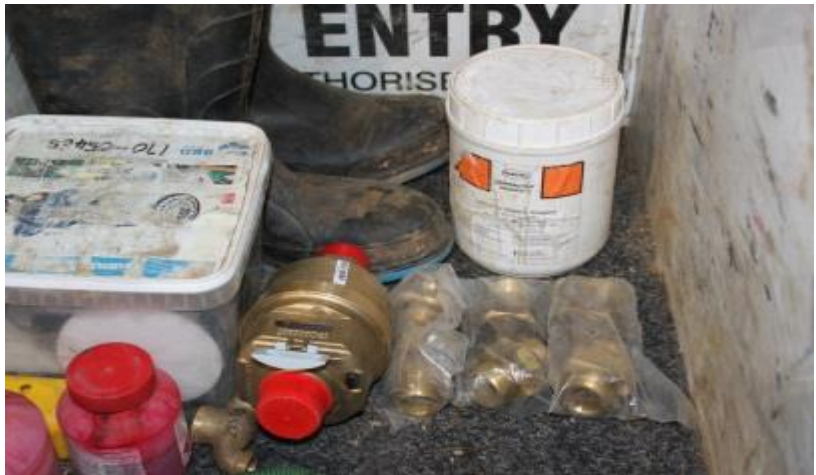
Fittings stored in a vehicle - note caps on meter, chemicals sealed and fittings in sealed bags
