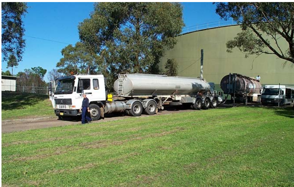
Figure 6 Static Collection and Mobile Disposal Tanker arrangement
